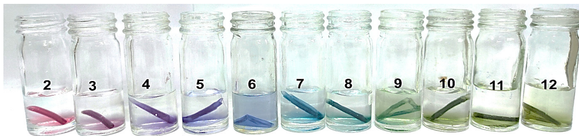
Fig. 3. Visual appearance of PS-BPE films in different buffer pH solutions (pH 2-12)
