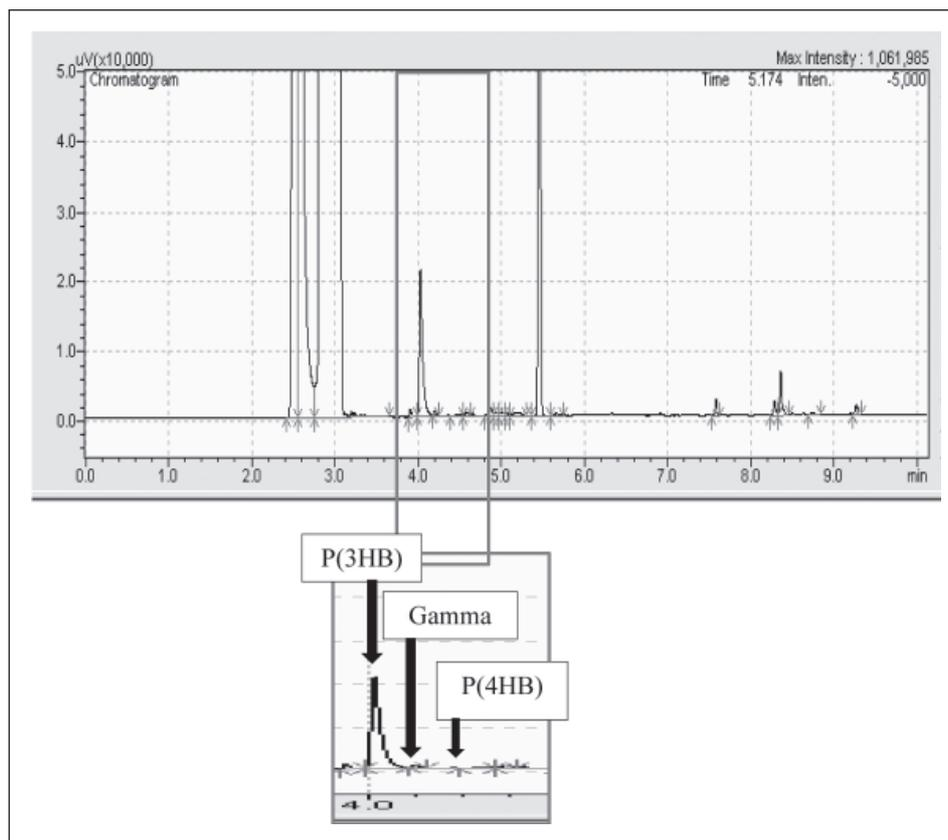
**Fig. 4.** GC analysis results showing the presence of copolymer P(3HB-co-4HB) in the bacteria isolate PD 16.
