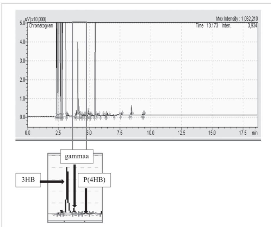
**Fig. 3.** GC analysis results showing the presence of copolymer P(3HB-co-4HB) in the bacteria isolate KPD 13.
