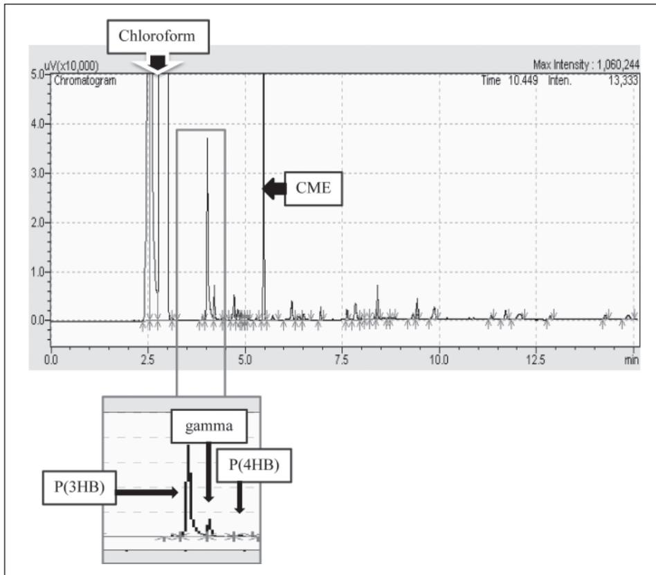
**Fig. 2.** GC analysis results showing the presence of copolymer P(3HB-co-4HB) in the bacteria isolate TMT 11.
