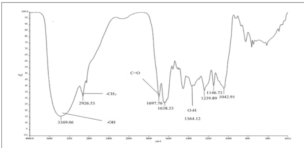
Fig. 2. IR spectrum of tea extracted with methanol.
