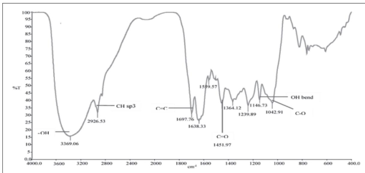
Fig. 1. IR spectrum of tea extracted with acetone.
