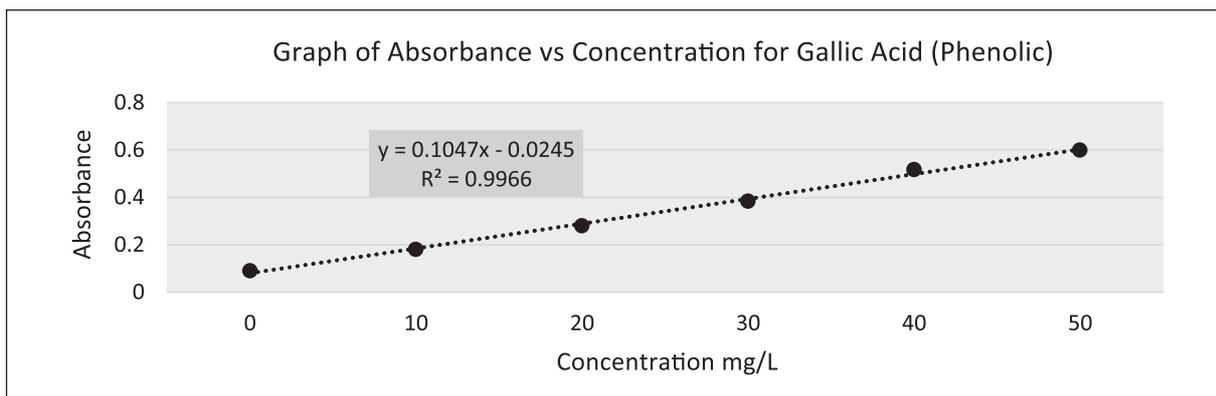
Fig. 5. Graph of absorbance vs concentration for Gallic Acid.
