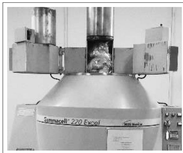
**Fig. 2.** Gamma Cell 220 Excel S.N. 117R cobalt-60 with banana *Mas* placed inside the chamber of Gamma cell.
